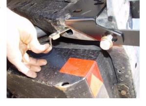
6. Insert 7/16"x1 1/2" bolt w/flat washer thru the bumper and lower strap, Thread on 7/16" Nylock w/flat washer. Do not tighten. Same on other side.
